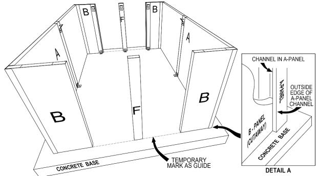
FIG. 1 NOTE: the "F" posts have been replaced with "B" (middle) panels, see the Enclosure Plan View.
