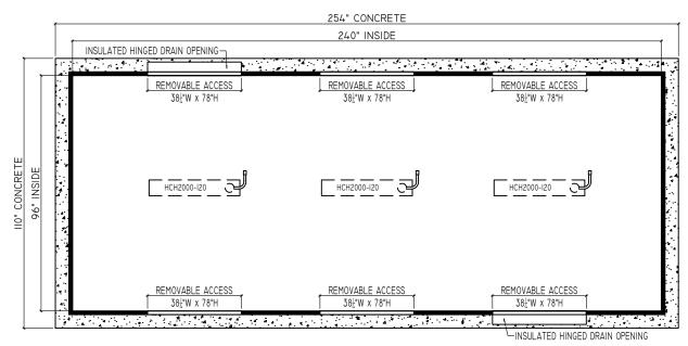
NOTE: ACCESS PANEL LOCATIONS CAN BE DETERMINED WHEN ENCLOSURE IS ORDERED. THIS MODEL RECEIVES UP TO 6 ACCESS PANELS AT THE SAME PRICE
