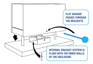
This puck lock on one side and flat washer on the opposite side are both flush to the enclosure, preventing would-be thieves or vandals with bolt cutters or hacksaws from breaking into your enclosure.
